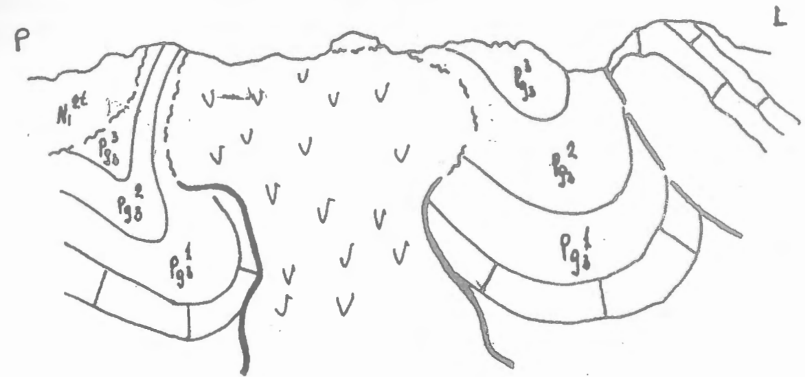
Fig.10 Profili skematik terthor ku paraqiten marredheniet e komplekseve shkembore me diapirin kripor ne variantin "shtok kripor". Indirect schematic Profil where are presented relations of the rocky complexions with salty diaper in "diaper salty" variant.
